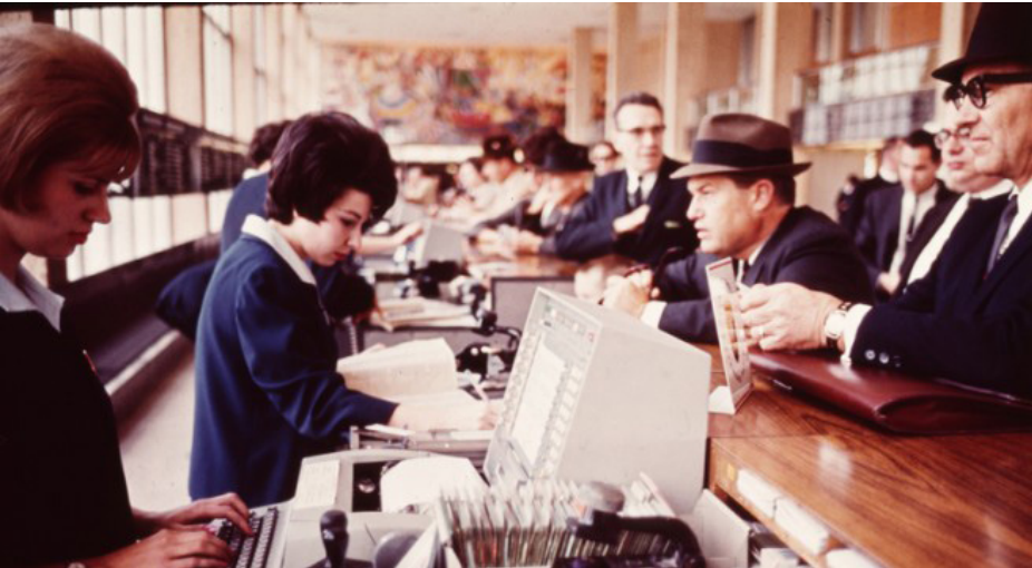
Below: The SABRE automated system reduced the time required to process a new airline reservation to just a few seconds. Image: IBM
